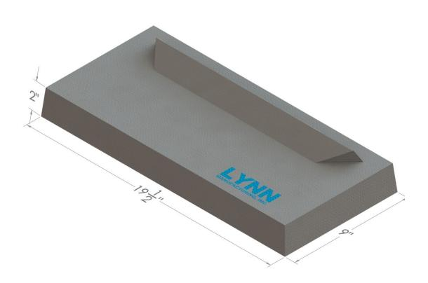
2303A REPLACES: Napoleon W010-3562 and old part number W018-0130. Sold as a single piece, complete replacement requires two pcs. This is the NEW thicker 2" baffle. Stoves built before 2010 may have a 4 piece baffle that can be replaced with two of these baffles
